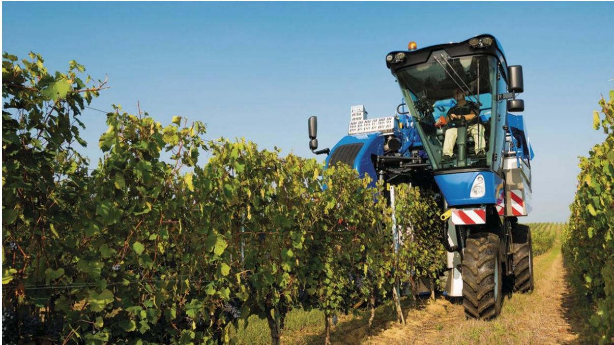
Vineyard grape ,mechanical harvester illustrating support structures (posts, wires etc)
